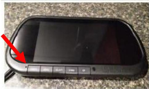
NOTE: If the monitor has power, the indicator to the left of the power button should be Blue when powered ON or Red when powered and in standby mode.
